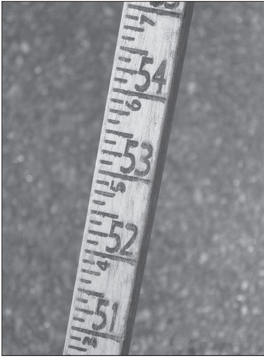
FIGURE 6-4. Verify that the numbers on the gauge stick are clear and easy to read and that the gauge stick is not warped or broken.
