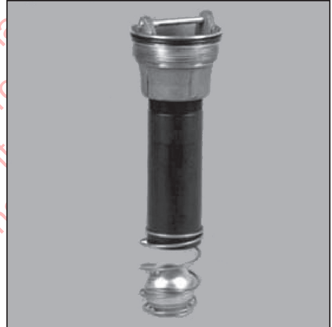
FIGURE 7-2. Ball float assembly showing the ball in the open position. The ball will float and cover the vapor path if the product rises above the level of the cage.
