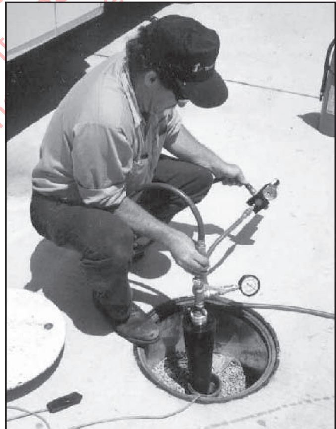
FIGURE 4-4. The plumber's plug provides a leak-tight connection to draw a vacuum on the tank interstitial space.
